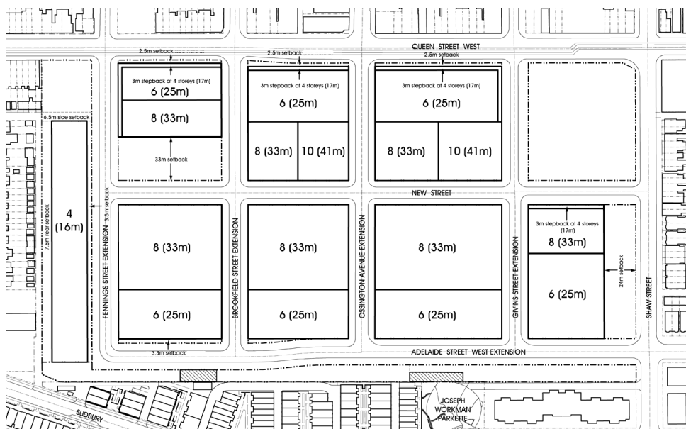
Proposed building envelopes (maximum heights in metres, also shown in storeys, and minimum setbacks) for the site.
